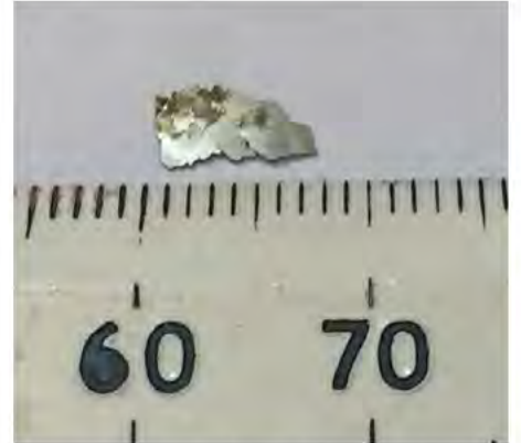
Above: The guilty fleck of flaked chrome, which was barely 8mm long and caused so much consternation!
